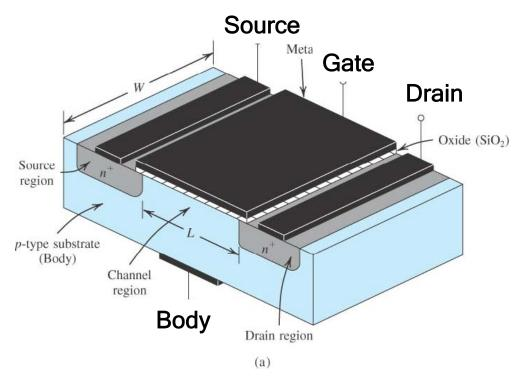
Control current flow between S and D with voltage applied at G NMOS, PMOS
