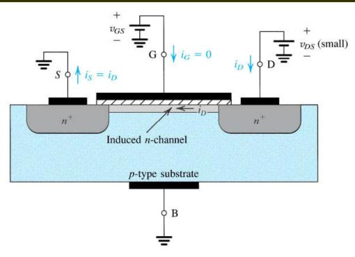
With  $v_{GS}>v_T$  (threshold voltage), channel is formed. (Gate and p-substrate is acting as a capacitor) More carriers with higher  $v_{GS}$
